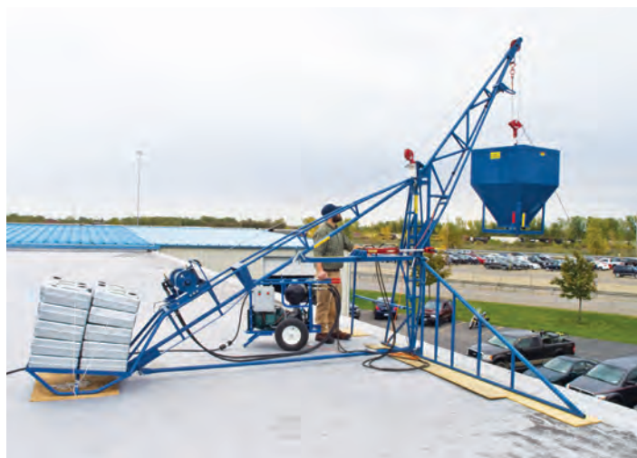
HS2000 Swing Hoist with 1600 lb. Gravel Bucket
